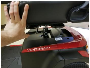
2. Place the removed seat aside. Now the shroud is exposed.
