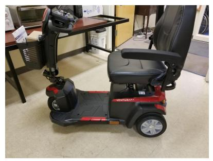
1. First step is to remove the seat. Pull up on the lever and lift to remove.
