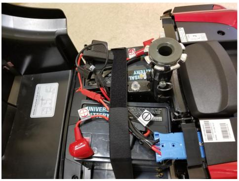
9. The batteries will need to be connected by these two plugs to get the unit running.
