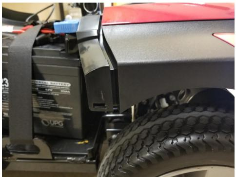
8. Note that the batteries will appear to be hooked up. You may need to plug in the blue cable on the left and white cable on the right.
