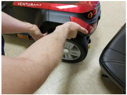
5. To remove, place pressure inward on the rear section, and pull outward and away on the front. This will cause the latch to disengage. (See step 8 for picture of latch)
